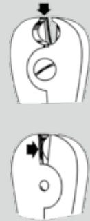
INS-23-5815-18T 18 cm / 7" for soft wires up to \varnothing 2 mm for hard wires up to \varnothing 1.5 mm
